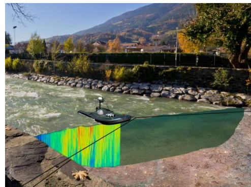
Figure 11:9 – RiverSurveyor M9 – Moving Boat Method
