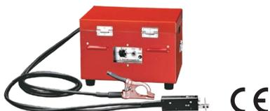
This is a spot welder used for installing weldable strain gauges and fixing leadwires. The welding energy is controlled in two ranges of 1~10 and 5~50 watt second. Its short welding pulse width of approximately 5 millisecond causes very little thermal damage on the material to be welded. The welding energy is not influenced by changes in the power source voltage owing to the adoption of stabilizing circuit. Electrical cables are stored inside the housing for convenience in field applications.
